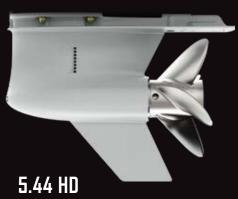
Designed to push heavy bay boats and multi-engine performance center console boats that require a more-submerged gearcase.
